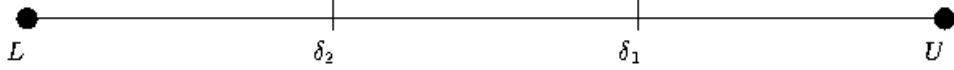
Figure 4.1: The trisection algorithm keeps track of an interval [L, U] containing \tau(A, B) . At each iteration either L is updated to \delta_2 or U is updated to \delta_1 .
