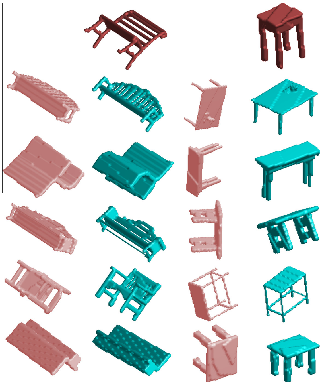
Fig. 14. Class-based ARR selection for bench seat and rectangular table classes. The top red figures are the reference models. Pink figures at the left are the outputs of CPCA-based normalization. Cyan figures under the reference models are the best choice out of the 48-ARR representations. (For interpretation of the references to color in this figure legend, the reader is referred to the web version of this article.)
