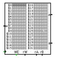
**Program ROM:** A 32-bit wide byte-addressed ROM, with built-in MIPS assembler. Use the attributes panel to load a MIPS assembly file into the ROM. The *PC* input specifies the address of the current instruction, and must be a multiple of 4. The output is the 32-bit instruction at the *PC* address, or zero if the *PC* has gone past the end of the ROM. Note that *zero* also happens to encode a no-op in MIPS. The assembly language is in the format described below.
