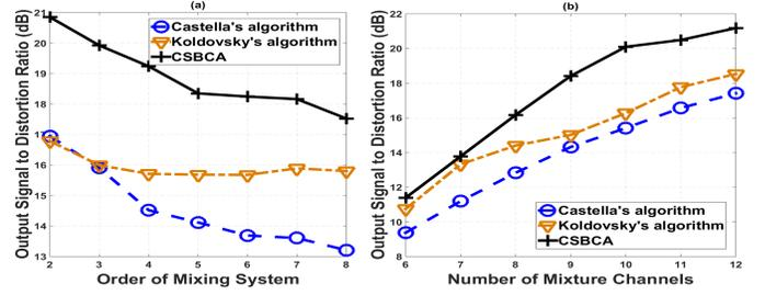
**Fig. 2.** a)- Output SDR vs. mixing order for 5 sources and 10 mixture channels under SNR=20 dB. b)- Output SDR vs. number of mixture channels for 5 sources under SNR=20 dB.
