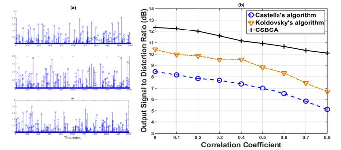
**Fig. 3.** a)- Copula-T distributed random sparse sequences. b)- Output SINR vs. correlation for 3 sources under SNR=20 dB.
