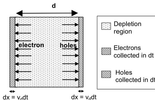
**Fig. 3** Modeling voltage time response through a charge flux calculation
