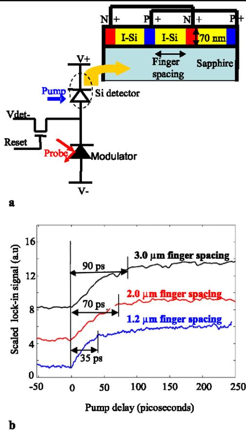
**Fig. 5** (a) Photodetector speed test—schematic of the structure under test, showing device connectivity (b) transient response for 1.2  $\mu\text{m}$ , 2.0  $\mu\text{m}$ , and 3.0  $\mu\text{m}$  finger spacing detectors
