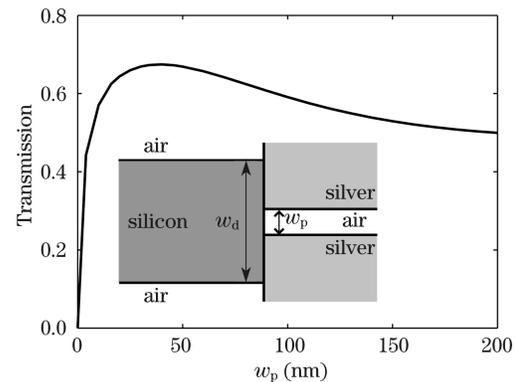
Fig. 5. Transmission efficiency of a coupler between a dielectric and a MDM waveguide as a function of the width of the plasmonic waveguide  $w_p$  at  $\lambda_0 = 1.55 \mu\text{m}$  calculated using FDFD. The coupler, created by placing the dielectric waveguide terminated flat at the exit end of the MDM waveguide, is shown in the inset. Results are shown for  $w_d = 300 \text{ nm}$ .
