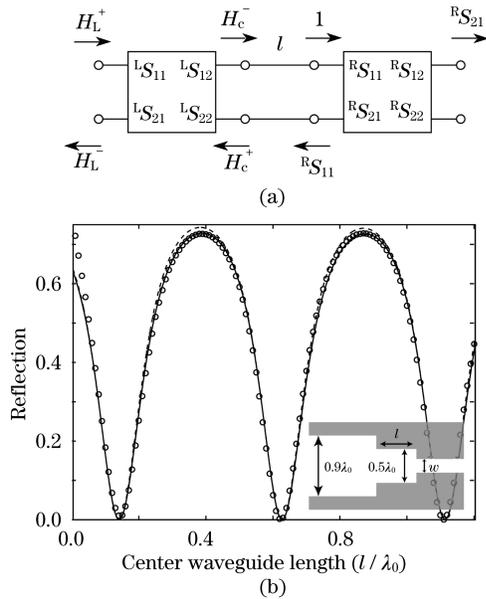
Fig. 3. (a) Schematic diagram of modal propagation. The left and right junctions are shown as boxes with an  $\mathbf{S}$  matrix description. The center waveguide is shown as a transmission line of length  $l$ . (b) Reflection coefficient for  $w = 0.16\lambda_0$  as a function of  $l/\lambda_0$  at  $\lambda_0 = 1.55 \mu\text{m}$  calculated using FDFD (circles). Transfer matrix calculations using lossy (solid line) and lossless (dashed line) junction models are also plotted.
