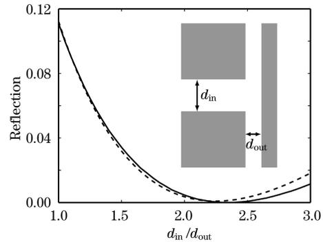
Fig. 2. Reflection coefficient  $R$  of a MDM T-shaped splitter (shown in the inset) as a function of  $d_{\text{in}}/d_{\text{out}}$  at  $\lambda_0 = 1.55$   $\mu\text{m}$  calculated using FDFD. We also show with dashed line the reflection coefficient  $\bar{R}$  calculated based on the characteristic impedance  $Z_{\text{MDM}}$  and transmission-line theory. Results are shown for  $d_{\text{out}} = 50$  nm.
