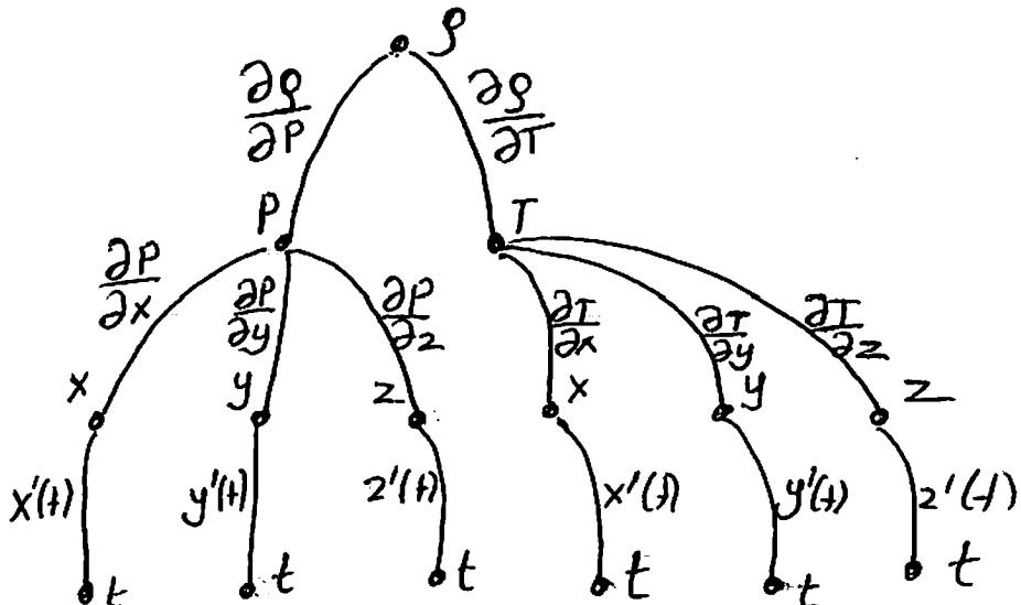
$$\frac{dg}{dt} = \underbrace{\frac{\partial g}{\partial P} \frac{\partial P}{\partial x} x'(t)}_{\text{Path through } P \text{ and } x} + \underbrace{\frac{\partial g}{\partial P} \frac{\partial P}{\partial y} y'(t)}_{\text{Path through } P \text{ and } y} + \underbrace{\frac{\partial g}{\partial P} \frac{\partial P}{\partial z} z'(t)}_{\text{Path through } P \text{ and } z}$$
