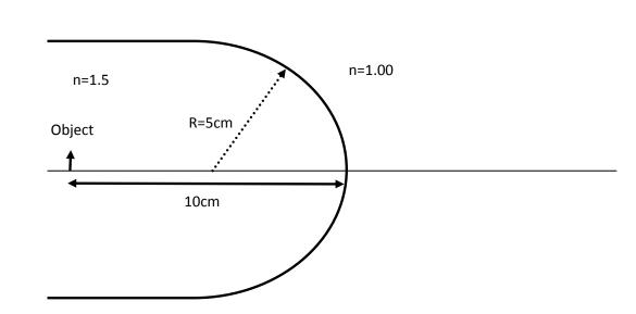
Hint: For refraction at a spherical surface  $\frac{n_a}{s} + \frac{n_b}{s'} = \frac{n_b - n_a}{R}$ .
