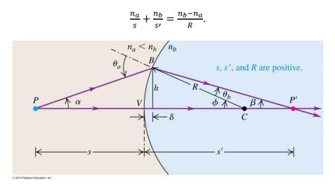
b) Find the ray transformation matrix corresponding to refraction at a spherical surface for rays transmitted from medium a to medium b, as shown above.
