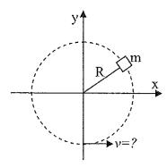
A particle of mass m suspended with a massless, unstretchable string of length R makes vertical circular motion. The speed of the mass is minimum at the highest point so as it barely swings through a complete vertical circle. (Gravitational acceleration is g)
