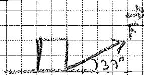
A farmer pulls a load a distance of 20m. The applied force is 5000N at an angle of  $37^\circ$  above the horizontal. There is a 3500N friction force opposing the load's motion.
