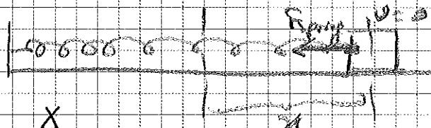
$$W_{\text{total}} = \int -kx \, dx = -\frac{1}{2} kx^2 = K_2 - K_1 = \frac{1}{2}mv_0^2 - \frac{1}{2}mv_1^2$$
