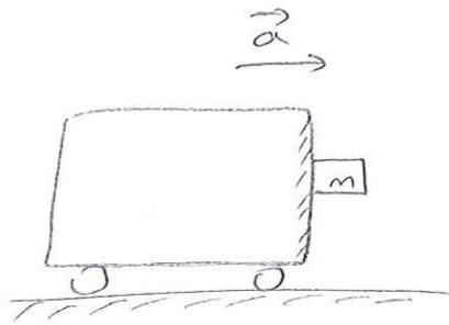
Friction force will resist the gravitational force.
