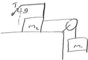
a) Tension in the rope accelerates the ball
