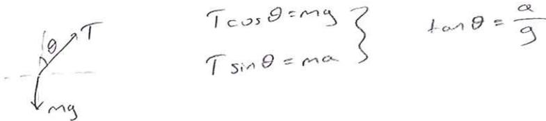
$$\left. \begin{aligned} T \cos \theta &= mg \\ T \sin \theta &= ma \end{aligned} \right\} \tan \theta = \frac{a}{g}$$
