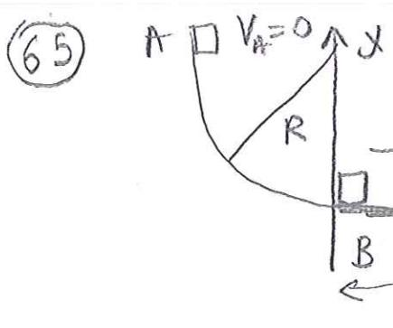
$$\begin{aligned} y_A &= R \\ y_B &= y_C = 0 \\ m &= 0,2 \text{ kg} \\ R &= 1,6 \text{ m} \\ d &= 3 \text{ m} \end{aligned}$$
