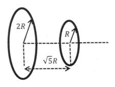
If m is placed in the center of 2R-ring:  $U_1 = -\frac{6Mm}{2R} + \frac{-6Mm}{6R} = \frac{-4.45}{4.30} \frac{6Mm}{R}$ It m is placed in the center of R-ring:  $u_2 = -\frac{GMm}{R} + \frac{-GMm}{7R} = \frac{-46Mm}{3R}$
