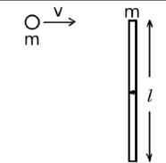
(a) Calculate (by integration) the moment of inertia *I* of the bar about its center.
