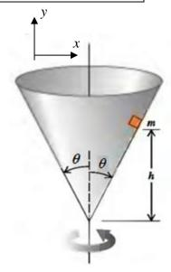
b.) Write the equations of Newton's  $2^{nd}$  law of motion in x and y directions.
