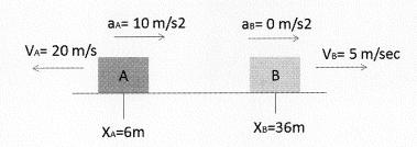
As shown in figure 1, two cars **A** and **B** move along the x –axis. **A** is travelling with a constant acceleration 10 m/sec2 and its initial velocity is 20 m/sec. The second car **B** is travelling with a constant speed of 5 m/sec. Pls note that their initial positions are also different.
