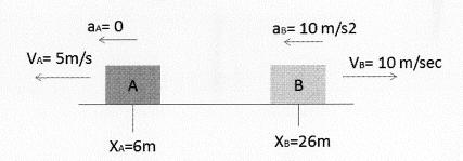
As shown in figure 1, two cars  $\bf A$  and  $\bf B$  move along the x –axis.  $\bf A$  is travelling with a constant velocity of 5 m/sec2. The second car  $\bf B$  is travelling with a constant acceleration of 10 m/sec2 and its initial velocity is 10 m/sec. Pls note that their initial positions are also different.
