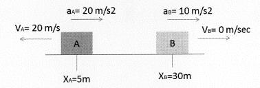
As shown in figure 1, two cars  $\bf A$  and  $\bf B$  move along the x –axis.  $\bf A$  is travelling with a constant acceleration 20 m/sec2 and its initial velocity is 20 m/sec. The second car  $\bf B$  is travelling with a constant acceleration of 10 m/sec. Pls note that their initial positions are also different.
