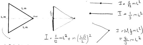
a) Calculate the total moment of inertia of the frame about the rotation axis through the pivot.
