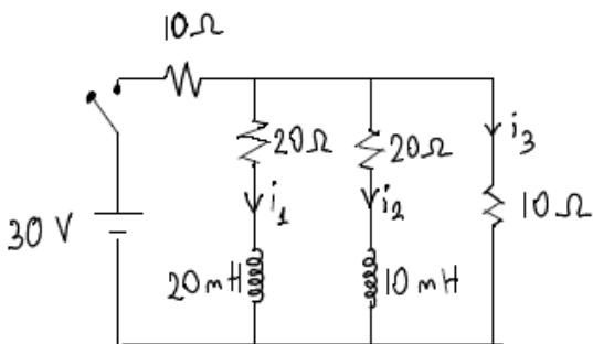
⑤ (a) At the initial moment inductors act like open switches. So we are dealing with an equivalent circuit as below
