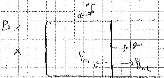
Work done by the force pulling the rod should be equal to the work of energy dissipation in the circuit.
