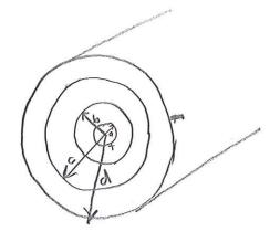
Assumption: Voltage is applied to the most inner and outer cylinders, having radius a and respectively.
