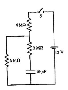
The capacitor is uncharged before the switch S is closed. So, it acts as a short circuit at the instant the switch S is closed. Circuit becomes
