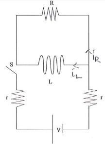
When switch Sis closed for a long time  $E_R \to 0$ .
