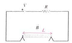
The Magnetic Force is given by  $F=ILB\sin\phi$  and  $F_I=mg$  when the bar is just ready to leviate. When I becomes larger,  $F_I>mg$  and  $F_I-mg$  is the net force that accelerates the bar upward.
