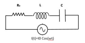
a) What is the resonance frequency *f* of the circuit in terms of Hz?
