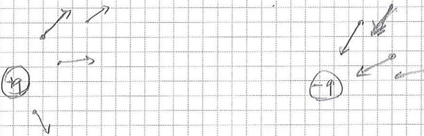
Electric field of a point charge points away from a positive charge but toward a negative charge ( $-\hat{r}$  direction)
