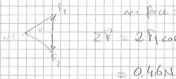
$$\text{net force: } \vec{F} = \vec{F}_1 + \vec{F}_2 = 2F_1 \cos 30^\circ = 2 \cdot 4 \cdot 9 \times 10^{-9} \frac{\text{Nm}^2}{\text{C}^2} \cdot \frac{2 \times 10^{-6} \text{ C}}{(0.3 \text{ m})^2}$$
