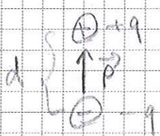
We define the electric dipole moment vector  $\vec{p}$ , as the vector with magnitude  $p = qd$  and direction from the negative charge.
