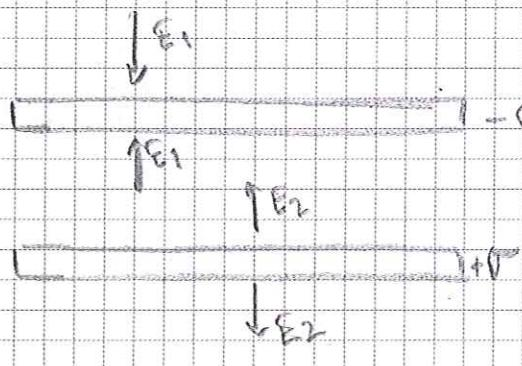
Two infinite parallel sheets are separated by a distance  $d$ .
