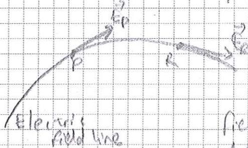
At any point, without a charge, the electric field has a unique direction, only one
