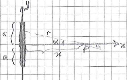
A charge  $Q$  is distributed uniformly along a line with length  $2a$ . What is the electric field on the axis along the middle of the line?
