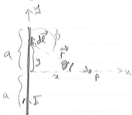
$\vec{B}$  at a point a distance  $r$  from the conductor on its perpendicular bisector.
