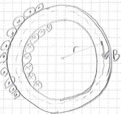
If the coils are very tightly wound, we can consider circular loops in the solenoid.
