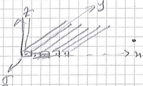
Long, straight conductors with square cross-sections each carrying current  $I$  are laid side-by-side to form an infinite current sheet.
