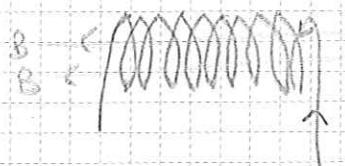
Field lines towards the center of a solenoid are nearly parallel.
