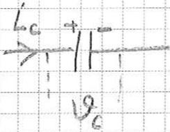
Choose the positive direction of current to be towards the + plate of the capacitor.
