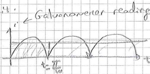
It is consisted of 4 diodes  $\Rightarrow$  these are elements which have 0 resistance in the forward and infinite resistance in the backward direction.
