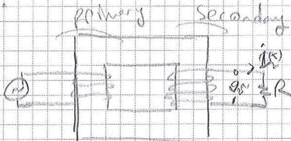
Two coils of different windings.
