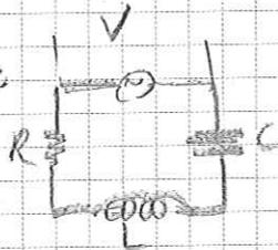
$R = 300\Omega$ ,  $L = 60\text{mH}$ ,  $C = 0.5\mu\text{F}$ ,  $V = 50\text{V}$ ,  $\omega = 1000\text{rad/s}$
