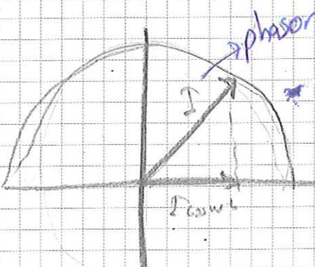
We use phasor diagrams to represent sinusoidally varying voltages and currents.
