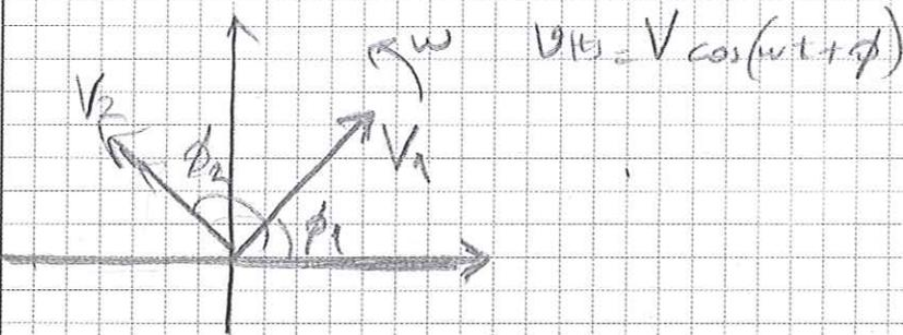
$$v_1(t) = V_1 \cos(\omega t + \phi_1) \quad , \quad v_2(t) = V_2 \cos(\omega t + \phi_2)$$
