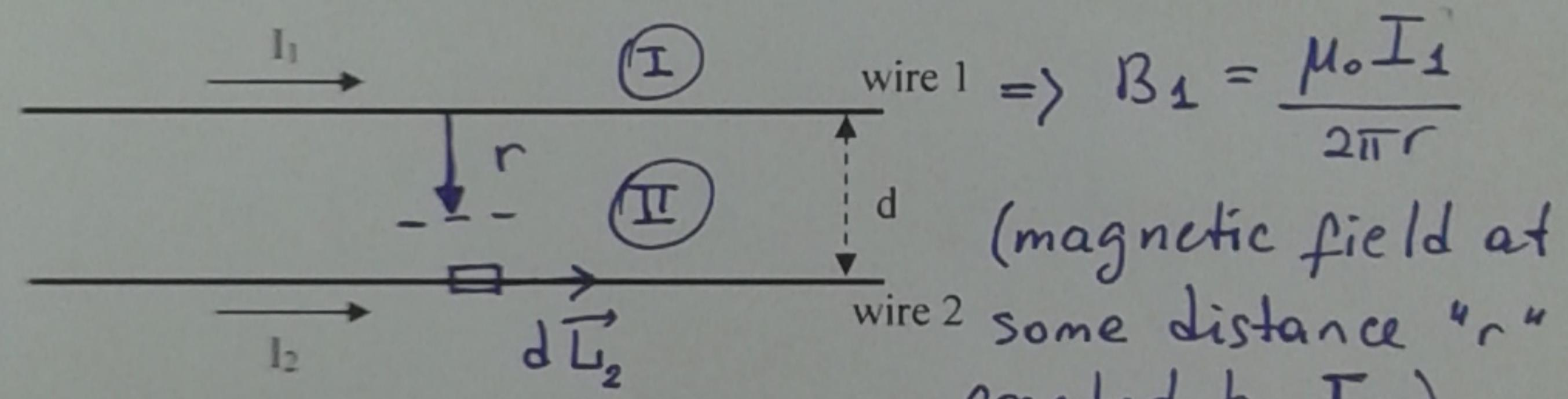
By the right-hand rule, the direction of  $\vec{B}_1$  in the region (II) is into the plane:  $\otimes \vec{B}_1$
