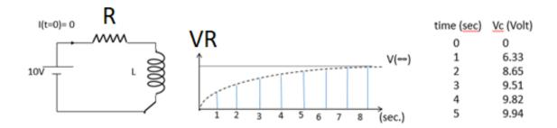
a) Calculate the time constant of the RL circuit using the graph given above.
