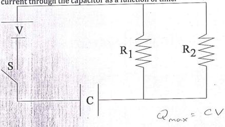
$$T = \frac{R_1 R_2 C}{R_1 + R_2}$$
