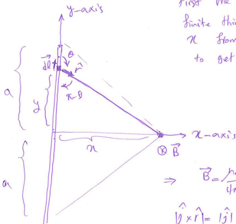
First we obtain the magnetic field of a finite thin wire with length  $2a$  in a distance  $x$  from its center. Then take  $a \rightarrow \infty$  to get the magnetic field of an infinite wire.
