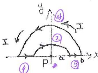
For parts ① and ③, because  $d\vec{l} \parallel \hat{r}$ , then  $\vec{B}_1 = \vec{B}_3 = \frac{\mu_0}{4\pi} \int \frac{I d\vec{l} \times \hat{r}}{r^2} = 0$
