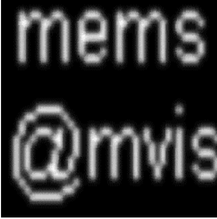
Figure 5: Simulated resultant display image at the center and the edge of the screen for the bidirectional scanning architecture shown in Figure 4. Text is 10pt Arial. K_{sp} is 1.0 in the horizontal axes and 1.2 in the vertical axes. The motion blur in the horizontal axis for a 100% pixel-duty-cycle is also taken into account (i.e. light is turned on at the beginning of the pixel time and kept on during the entire pixel time).
