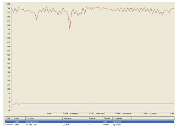
Fig. 8. Run-time cost of the P2P application: measured parameters are CPU idle time (upper line) and UDP bytes per second (lower line).
